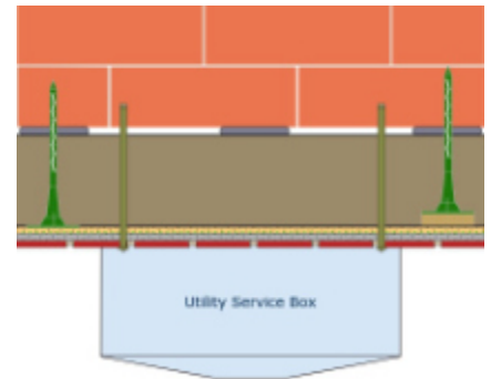
Detail 46 - surface mounted utility boxes
